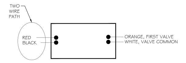
Decoder Wiring - SLDEC1
