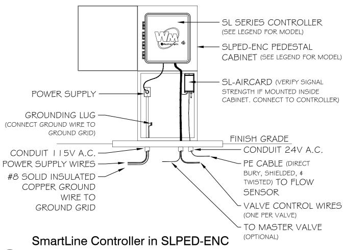
Enclosure with SLW & Aircard with Flow
