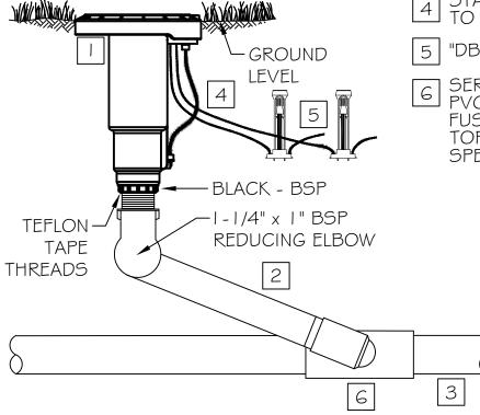
D50E / 55E WITH PVC / HDPE SWING JOINT - BSP
