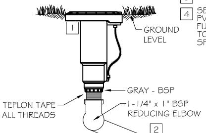
SERVICE TEE OR END ELBOW - PVC, HDPE SADDLE, OR HDPE FUSION CONNECTION. MAY BE TOP OUTLET. SEE DESIGNER'S SPECIFICATIONS.
